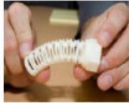
SLS Flex Cord passed 20,000 flexes without fracturing.
