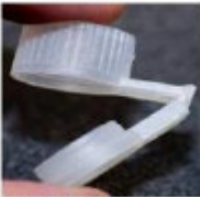
SLA fully functional pop design living Hinge picture on left for medical application. Standard living hinge pictured on right.
