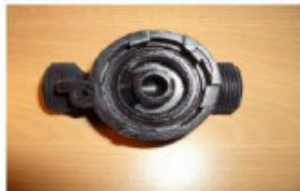
FDM ABS Pump Housing for weed control chemical had to be fully functional with 175psi vacuum pressure.
