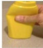
SLA fully functional squeezable bottle for mustard. This bottle passed the life cycle fatigue test in ambient and refrigerated temperature when squeezing out mustard and holding the fluids.
