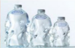
SLA Bottles to hold Chemical Reagent. Lids were tightened down and chemical do not leak or sweat after two months of life cycle fatigue test.
